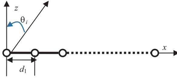
Figure 1. Geometry of antenna array.
