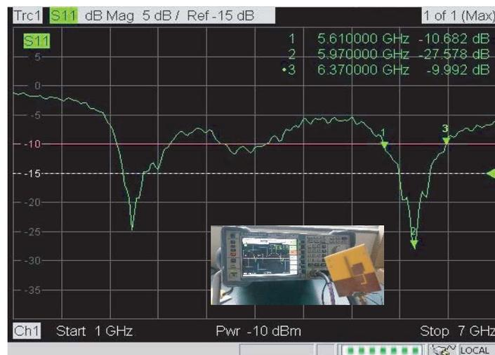
**Figure 17.** Measured return loss and experimental setup.
