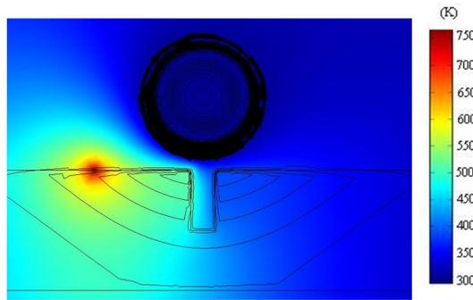
**Figure 4.** The diffusion of heat from laser beam and eddy current density distributions. EC frequency, 600 kHz; laser temperature, 500°C (773 K).
