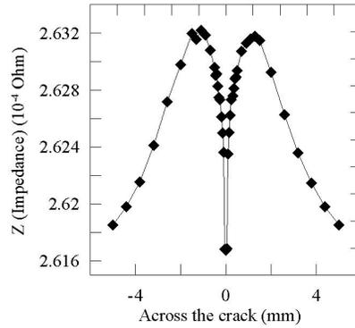
**Figure 6.** The flaw impedances of PI signal for a 0.5-mm rectangular notch in Ti-6Al-4V. EC frequency, 600 kHz; laser temperature, 300°C.
