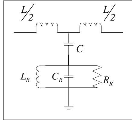
**Figure 2.** Equivalent lumped parameter circuit of CSRR.
