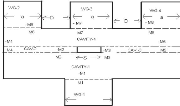
**Figure 2.** Cavity modeling and details of a basic 1:3 power divider.
