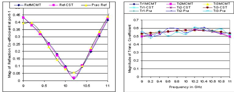
**Figure 3.** Comparison of theoretical, CST Microwave Studio simulated and measured data for an  $H$ -plane 1:3 WR-90 waveguide power divider with  $2t = 19.5$  mm.
