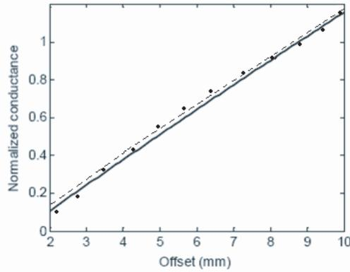
**Figure 3.** Normalized conductance as a function of slot offset. Solid line: computed, dashed line: simulated, dotted line: measured results. Dimensions are:  $2a = 22.86$ ,  $2b = 10.16$ ,  $t = 1.27$ ,  $2L = 16$ ,  $2w = 1$  mm.
