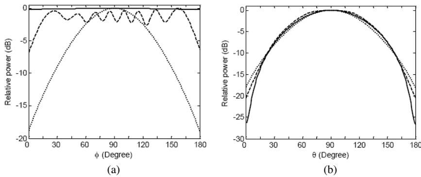
**Figure 6.** (a)  $E$  and (b)  $H$ -plane radiation patterns of a broad wall longitudinal slot for offset = 6 mm. Solid line: computed, dashed line: simulated with extended ground plane and dotted line: simulated with finite ground plane. Dimensions are:  $2a = 22.86$ ,  $2b = 10.16$ ,  $t = 1.27$ ,  $2L = 16$ ,  $2W = 1$  mm.
