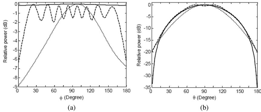
**Figure 5.** (a)  $E$  and (b)  $H$ -plane radiation patterns of a broad wall longitudinal slot for offset = 3 mm. Solid line: computed, dashed line: simulated with extended ground plane and dotted line: simulated with finite ground plane. Dimensions are:  $2a = 22.86$ ,  $2b = 10.16$ ,  $t = 1.27$ ,  $2L = 16$ ,  $2W = 1$  m.
