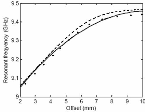
**Figure 4.** Resonant frequency as a function of slot offset. Solid line: computed, dashed line: simulated, dotted line: measured results. Dimensions are:  $2a = 22.86$ ,  $2b = 10.16$ ,  $t = 1.27$ ,  $2L = 16$ ,  $2w = 1$  mm.
