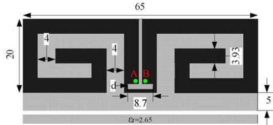
**Figure 1.** Geometry of the proposed printed dipole antenna.
