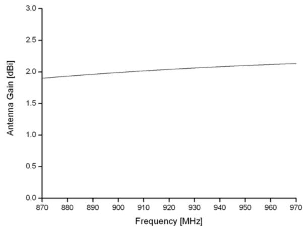
**Figure 7.** Measured gain of the proposed antenna.
