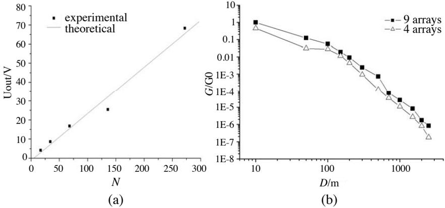
**Figure 6.** Axis field component synthesis of different number sub-arrays. (a) Axis field component at distance of 100 m, (b) 4, 9 sub-array axis energy at the same condition.
