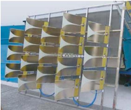
**Figure 3.** Antenna array.
