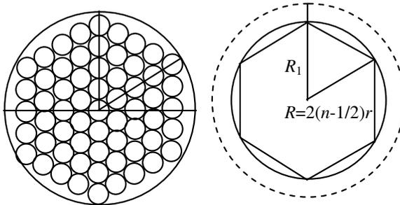
**Figure 2.** Fibers arranged as hexagon.
