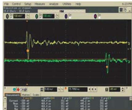
**Figure 4.** Transient electromagnetic pulse at the distance of 100 m.
