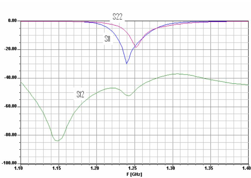
Figure 4. Return loss at L-band frequencies.
