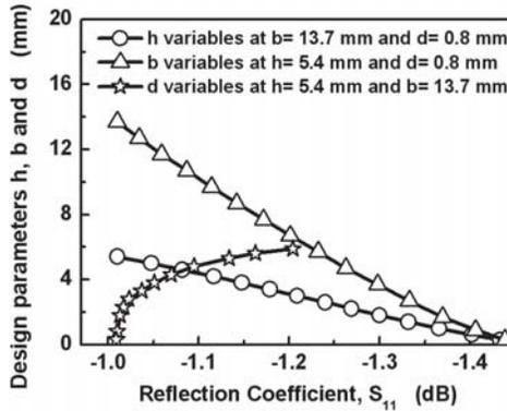
**Figure 4.** Reflection coefficient ( $S_{11}$ ) of EBG CPW by varying the design parameters ( $h$ ,  $b$ , and  $d$ ).
