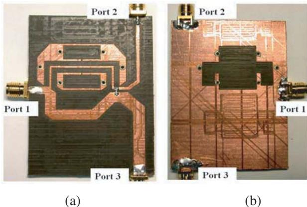
**Figure 6.** Photograph of the fabricated 6:1 Wilkinson power divider (a) top side, (b) bottom side.
