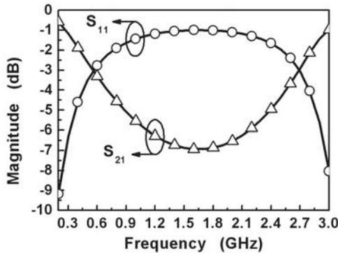
**Figure 5.** Electromagnetically calculated  $S$ -parameter of the proposed EBG CPW.
