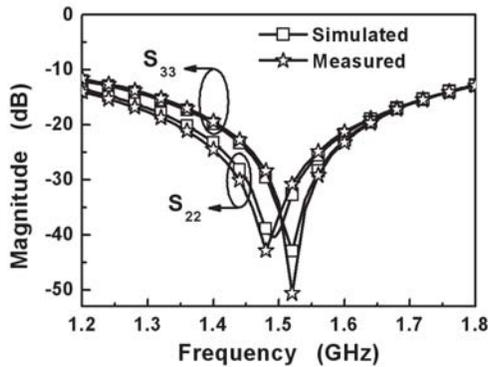
**Figure 8.** The simulated and measured results of the output return loss as a function of frequency.
