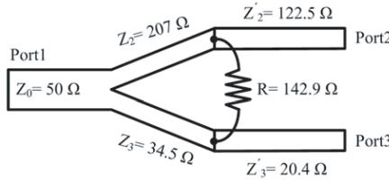
**Figure 1.** Topology of a 6:1 unequal Wilkinson power divider including its parameters.
