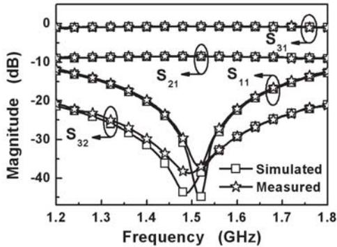
**Figure 7.** The simulated and measured results of the insertion loss, isolation, and input return loss as a function of frequency.
