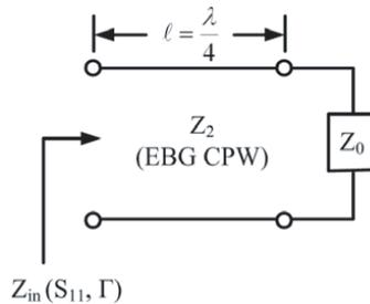
**Figure 3.** Simplified model to determine the characteristic impedance ( $Z_2$ ) of EBG CPW.
