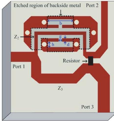
**Figure 2.** A schematic diagram of the proposed 6:1 unequal Wilkinson power divider.
