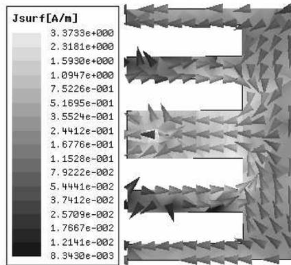
**Figure 7.** Current distribution at 2.18 GHz.
