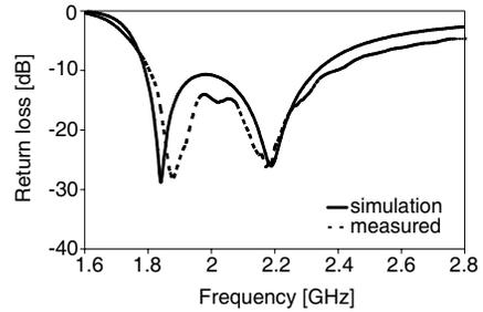
**Figure 3.** Return loss of the proposed patch.
