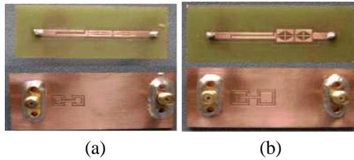
**Figure 5.** Fabricated proposed BPFs. (a) Type 1. (b) Type 2.
