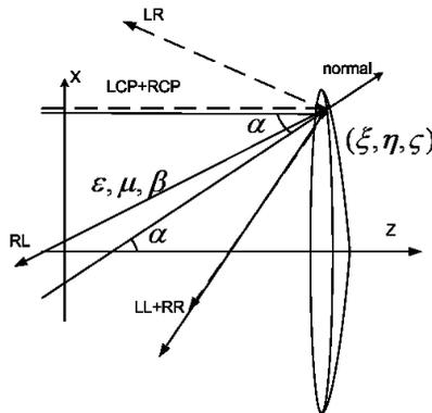
Figure 3. PEMC paraboloidal reflector placed in chiral medium.
