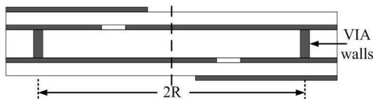
**Figure 2.** Side view of HSICC and SICC resonators.
