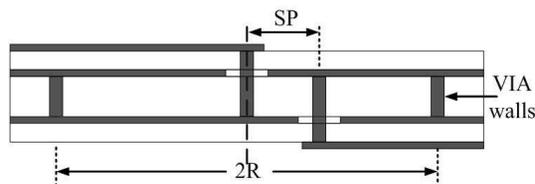
**Figure 6.** Side view of feeding structure using probes excitation.
