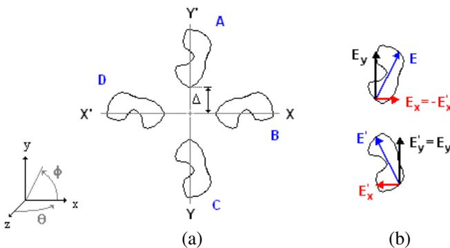
**Figure 1.** (a) Structure of clover array in coordinate system; (b) Electric field vectors ( $E$  and  $E'$ ) radiated from single elements of sub-array and their decompositions in  $x$  and  $y$  components.
