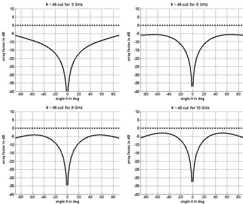
**Figure 3.** Comparison of theoretical cross-polarisation pattern of single antenna (dotted) and CA with the same source current (solid). The cut is made for  $\phi = 45^\circ$ .
