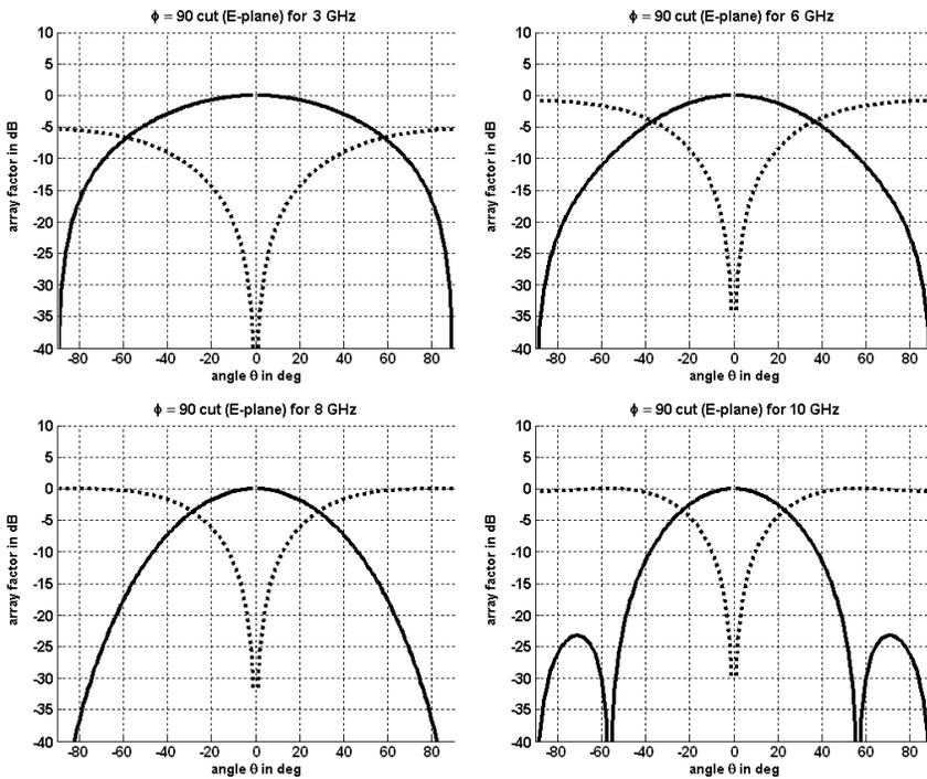
**Figure 2.** Theoretical array factor of the clover array for different frequencies. Solid line: co-polarisation, dotted: cross-polarisation.
