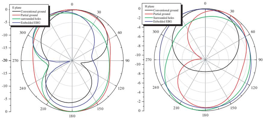
**Figure 14.** The measured  $E$ -plane and  $H$ -plane radiation pattern for MPPA at higher frequency (12 GHz).
