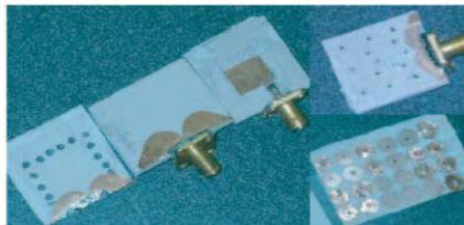
**Figure 12.** The fabricated of the proposed antennas without and with EBG structures.
