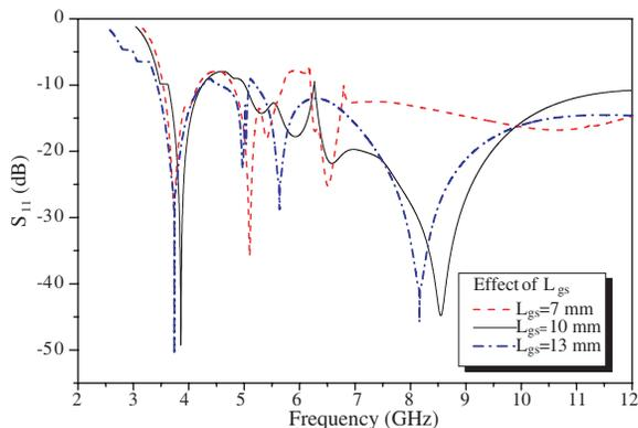
Figure 5. Effect of the  $L_{gs}$  of the MGP.
