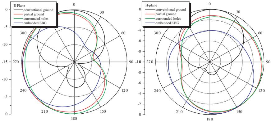
**Figure 13.** The measured  $E$ -plane and  $H$ -plane radiation pattern for MPPA at lower frequency (2.5 GHz).
