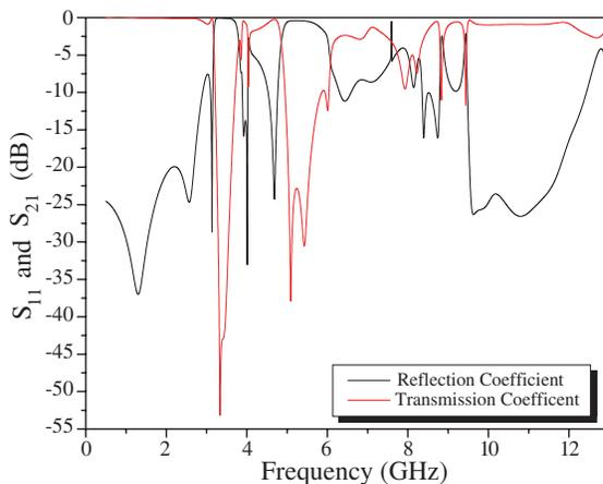
**Figure 8.** Transmission and reflection coefficient of the embedded circular patches.
