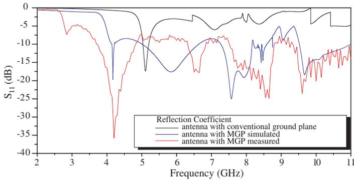
**Figure 6.** The comparison between simulated and measured of the reflection coefficient of the proposed antenna.
