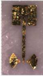
Figure 8. Microphotograph of the patch antenna.
