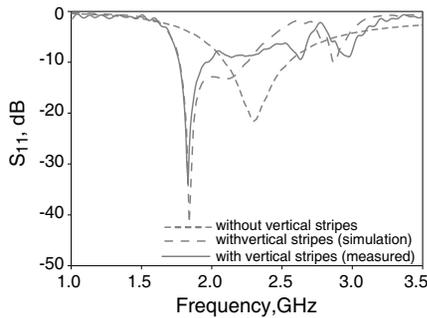
**Figure 2.** Return loss characteristics of the antenna.
