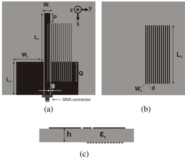
**Figure 1.** Geometry of the proposed antenna (a) 3D schematic diagram, (b) bottom view, (c) side view ( $L_1 = 25$  mm,  $W_1 = 3$  mm,  $L_2 = 17$  mm,  $W_2 = 14$  mm,  $g = 0.35$  mm,  $L_3 = 30$  mm,  $W_3 = 0.3$  mm,  $d = 0.5$  mm,  $h = 1.6$  mm,  $\epsilon_r = 4.4$ ).
