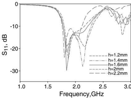
**Figure 7.** Variation of  $S_{11}$  with substrate height ( $h$ ).
