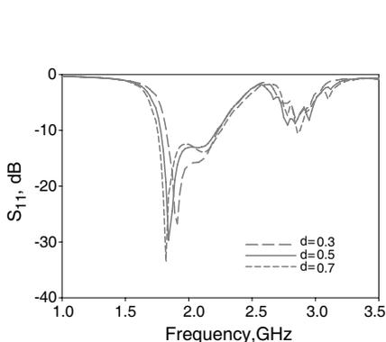
**Figure 9.** Variation of  $S_{11}$  with separation between the stripes.
