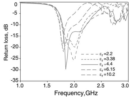
**Figure 6.** Variation of  $S_{11}$  with different substrate.
