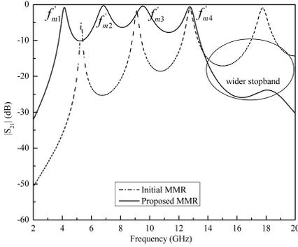
**Figure 6.**  $|S_{21}|$  comparison of initial and proposed MMR.
