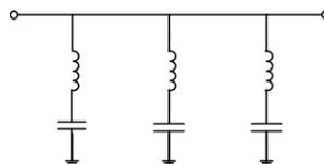
**Figure 5.** Equivalent circuit model of the proposed MMR.
