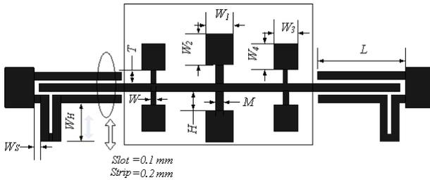
**Figure 1.** Schematic of the proposed UWB BPF.
