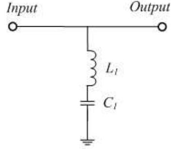
**Figure 7.** Equivalent circuit of the folded arm.
