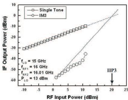
**Figure 7.** Intermodulation characteristics of the CMOS IRM.
