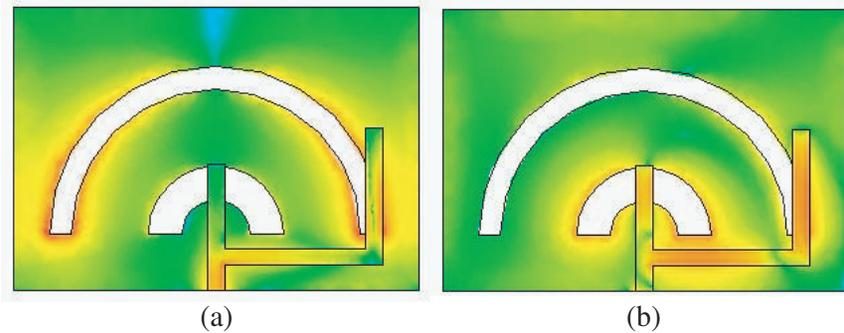
**Figure 5.** The surface current distribution at (a) 2.45 GHz; (b) 5.5 GHz.
