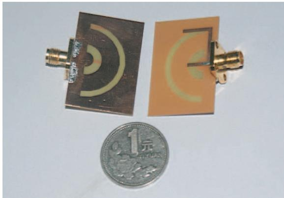
Figure 6. Photograph of the proposed antenna.
