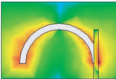
**Figure 3.** The surface current distribution fed by edge feeding method.
