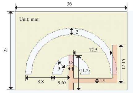
**Figure 4.** Configurations of the proposed antenna.
