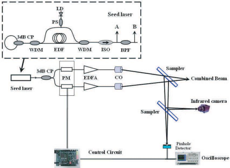
**Figure 1.** Experimental setup for phase locking of ultrabroad linewidth fiber amplifiers. LD: 974 nm pump laser diodes. PS: Power splitter. WDM: Wavelength-division multiplexer; EDF: Erbium doped fiber. CP: Coupler. ISO: Isolator. BPF: Bandpass filter. PM: Phase modulator. EDFA: Erbium doped fiber amplifier. CO: Collimator. A and B: The points where the laser power and spectrum is to be measured.
