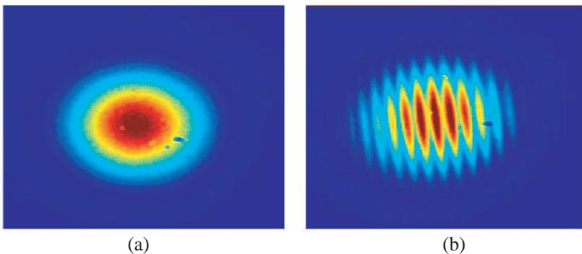
**Figure 3.** Long-exposure far-field intensity distributions: (a) Open loop without active phase control; (b) Close loop with active phase control.
