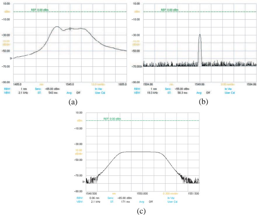
**Figure 2.** Optical spectrums. (a) ASE spectrum. (b) Filtered ASE spectrum. (c) Enlarged version of (b).
