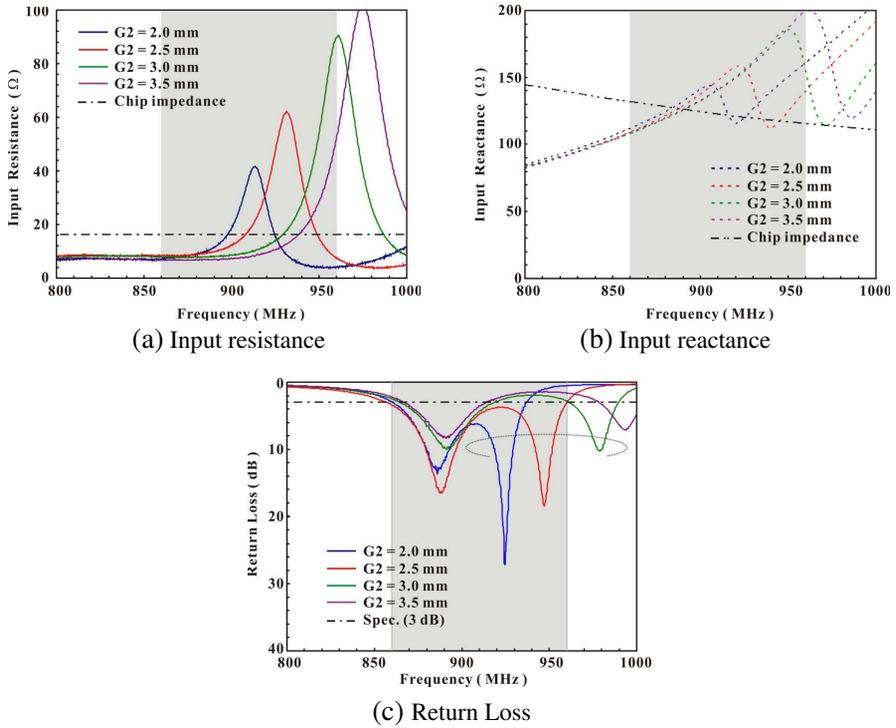
**Figure 7.** Measured impedance and return loss for the proposed F-shaped tag antenna with various gaps between the closed loop and the parasitic strip 2; other antenna parameters are given in Table 1.
