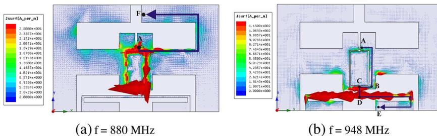
**Figure 3.** Simulated surface current distributions for the proposed F-shaped tag antenna.
