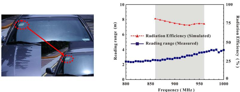
(a) Tag mounted on the automotive front glass (b) Reading range and radiation efficiency
