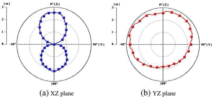
**Figure 8.** Measured XZ plane and YZ plane reading range patterns for the proposed planar tag antenna operating at 925 MHz.
