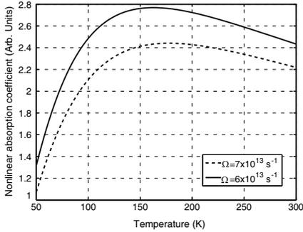
**Figure 3.** Dependence of  $\alpha$  on  $T$  at different values of  $\Omega$ .
