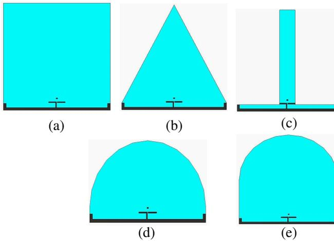
**Figure 4.** Different shapes of the substrate, (a) Rectangle, (b) Triangle, (c) T shape, (d) Semicircle, (e) Dome.
