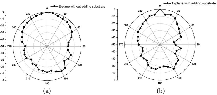
**Figure 9.** The measured results of radiation pattern in  $E$ -plane. (a)  $E$ -plane without adding substrate. (b)  $E$ -plane with adding substrate.
