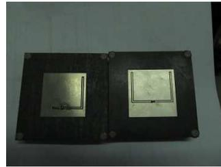
**Figure 12.** Photograph of the two proposed antennas.
