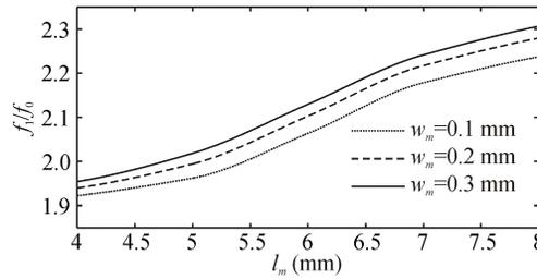
**Figure 4.** Three sets of frequency ratios of the two passbands versus the lengths of the microstrip lines ( $l_m$ ). ( $r_1 = 8.24$  mm,  $r_2 = 8.26$  mm,  $w_m = 0.30$  mm,  $w_s = 0.20$  mm,  $l_s = 2.5$  mm).
