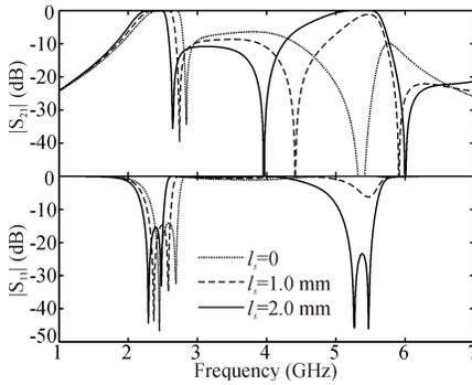
**Figure 2.** Frequency responses of  $S$ -magnitudes under varied stub lengths ( $l_s$ ). Substrate  $\epsilon_r = 10.8$ , thickness = 1.27 mm.  $r_1 = 8.24$  mm,  $r_2 = 8.26$  mm,  $w_m = 0.30$  mm,  $l_m = 7.0$  mm,  $w_s = 0.20$  mm.
