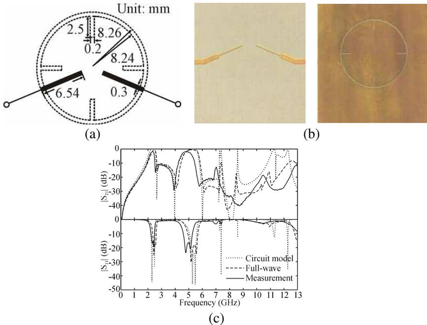
**Figure 5.** (a) Physical layout of the designed filter. (b) Photograph of the fabricated filter. (c) Circuit and EM simulated and measured frequency responses.
