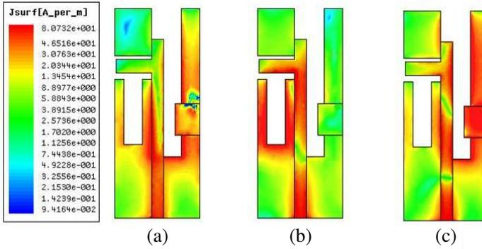
**Figure 5.** Surface current distribution at different frequencies. (a) 2.44 GHz. (b) 3.5 GHz. (c) 5.8 GHz.
