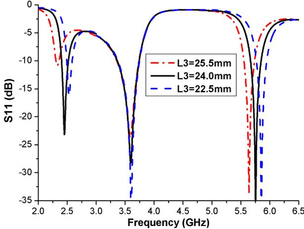
**Figure 6.**  $S_{11}$  variations for different values of slot's length  $L_3$ .
