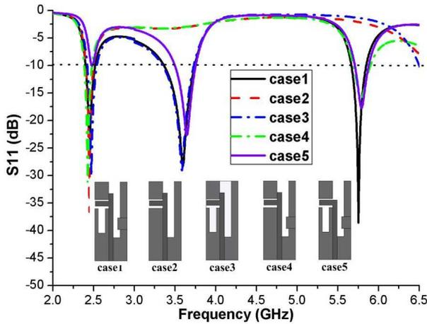
**Figure 4.**  $S_{11}$  variations of the proposed antenna in the different cases.
