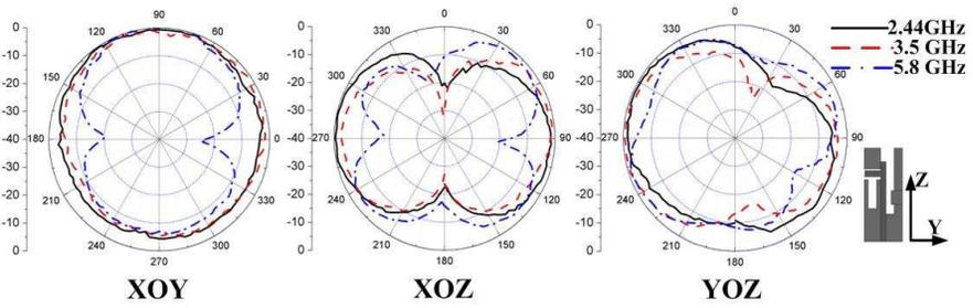
**Figure 9.** Radiation patterns in main cut planes.
