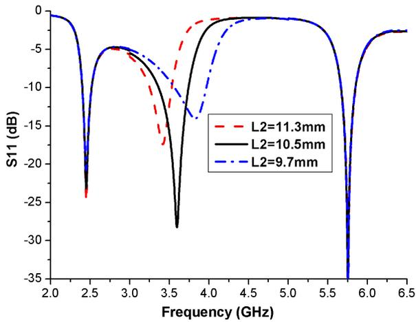
**Figure 7.**  $S_{11}$  variations for different values of slot's length  $L_2$ .
