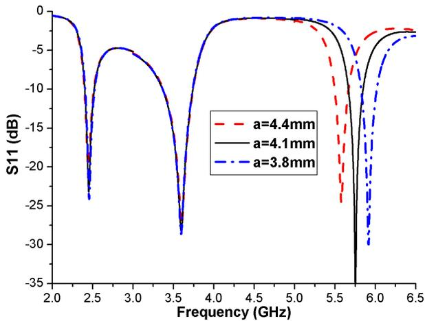
**Figure 8.**  $S_{11}$  variations for different values of square patch's width  $a$ .
