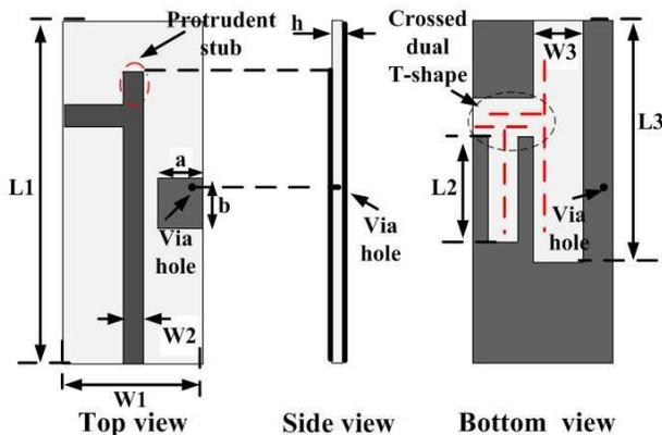
**Figure 1.** Geometry of the proposed triple-frequency slot antenna.
