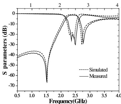
**Figure 5.** Simulated and measured results of the proposed filter.
