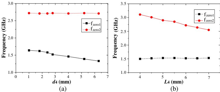
**Figure 4.** Transmission zero characteristic of the proposed filter (a) with  $L_4 = 6$  mm and (b) with  $d_4 = 2.8$  mm.
