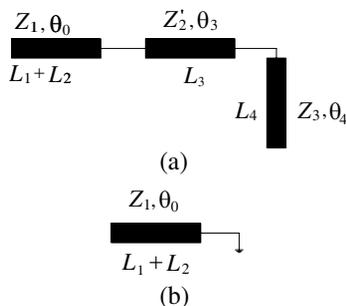
**Figure 3.** Equivalent circuit at (a) even mode, and (b) odd mode.
