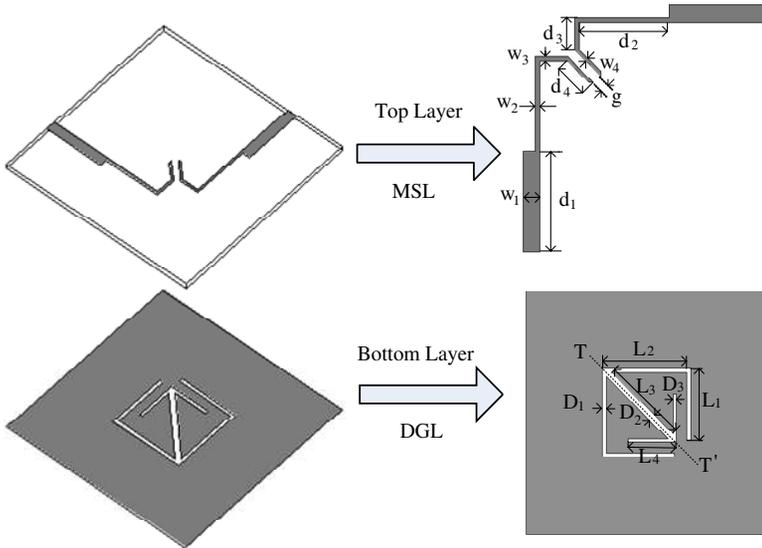
**Figure 1.** Configuration of the defected ground open-loop filter.
