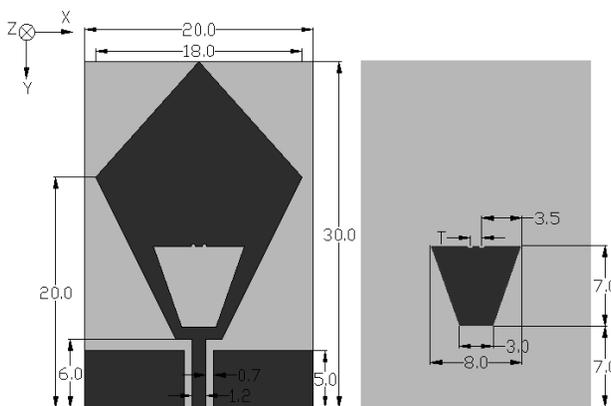
**Figure 1.** Geometry and dimensions of proposed antenna (mm).
