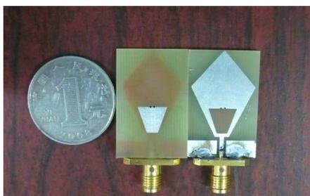
**Figure 3.** Photograph of the manufactured band-notched antenna.
