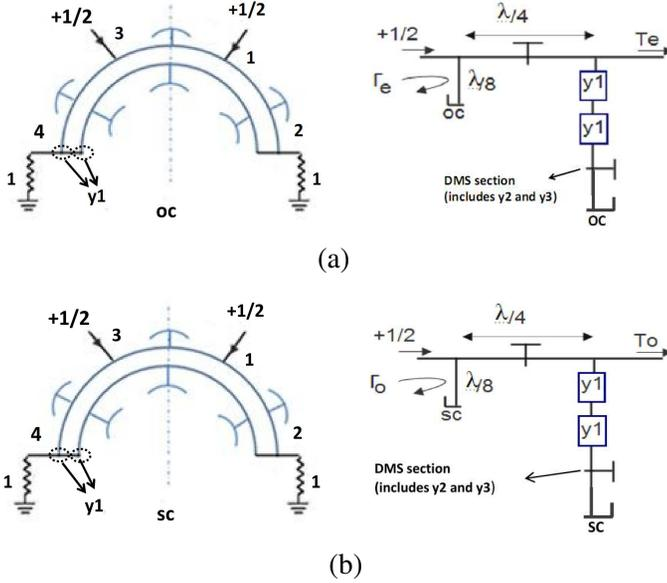
**Figure 7.** Equivalent topologies of the proposed rat-race coupler for (a) even and (b) odd excitations.
