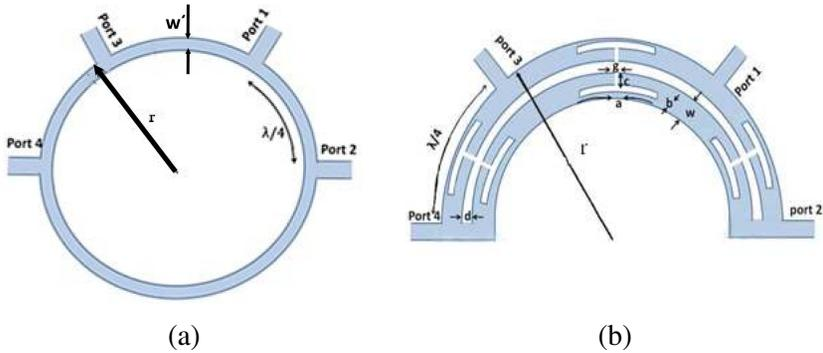
**Figure 1.** (a) Lay-out of the conventional rat-race hybrid ring and (b) Layout of small size ring coupler for symmetrical feeding ports with DMS ( $a = 13.68$  mm,  $b = 0.9$ ,  $c = 1.5$  mm,  $g = 0.4$  mm,  $d = 0.4$  mm,  $r = 21$  mm,  $w = 3$  mm and  $w' = 1.2$  mm).
