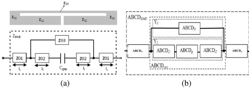
**Figure 4.** (a) A simple DMS circuit model with  $l_1 = 3.16$  mm,  $l_2 = 6.64$  mm, and  $C_{gap} = 0.03$  pF and (b) ABCD configuration of a DMS Section model.
