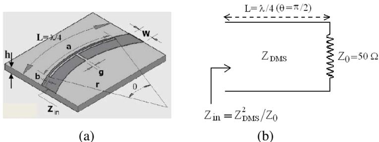
**Figure 2.** (a) Curved DMS Section ( $a = 13.68$  mm,  $b = 0.9$  mm,  $c = 1.5$  mm and  $g = 0.4$  mm) and (b) simplified model for the microstrip line with the DMS.
