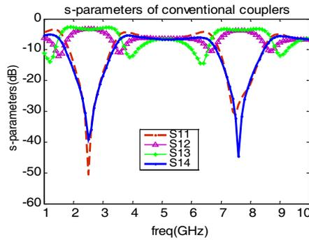
**Figure 11.** Simulation result of the conventional rat-race ring coupler with 70.7 ring impedance.
