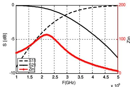
**Figure 3.** Matlab results of the microstrip line with the DMS section.
