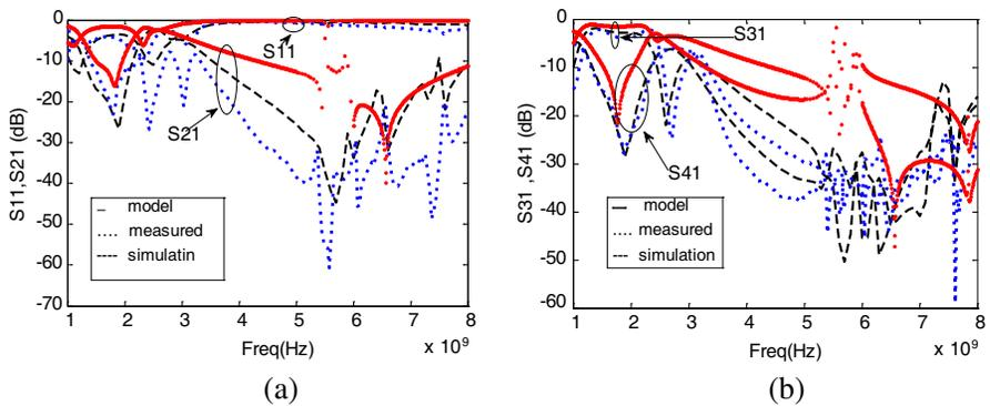
**Figure 10.** Performance of the rat-race coupler designed at  $f = 1.7$  GHz. (a)  $S_{11}$  and  $S_{21}$  and (b)  $S_{31}$  and  $S_{41}$ .
