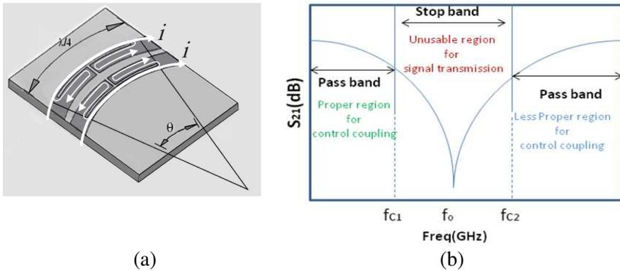
**Figure 5.** (a) A part of transmission line of proposed rat-race and relationship between maximum current paths and (b) investigation of different region of DMS transmission line frequency response.
