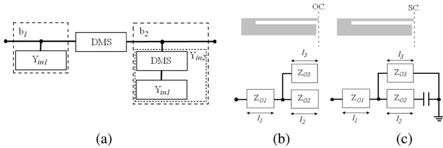
**Figure 9.** (a) ABCD configuration of the equivalent topologies of the proposed rat-race coupler, Branch line model  $Y_{in1}$  equivalent for (b) even and (c) odd excitations.
