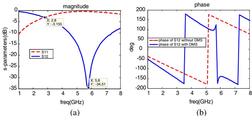
**Figure 6.** Simulation result of the microstrip line with the DMS section (a)  $S$ -parameters and (b)  $S_{12}$  phase.
