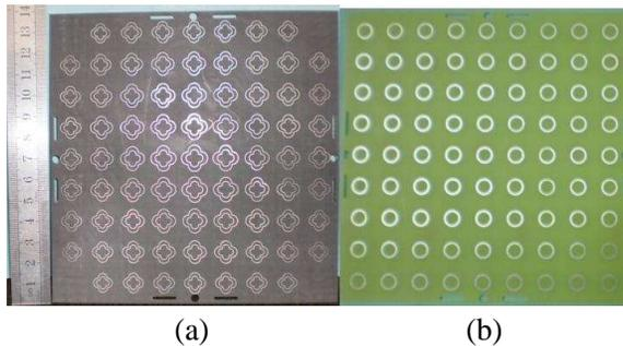
**Figure 7.** Photograph of the designed 77-element reflectarray and 81-element FSS ground.
