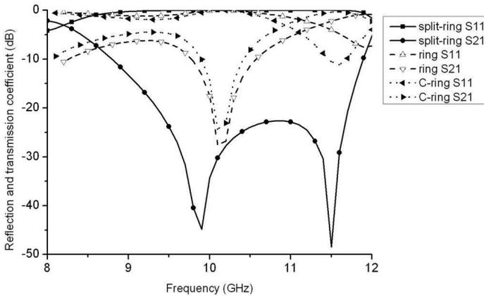
**Figure 4.** Reflection and transmission coefficients of the three types of FSS elements.
