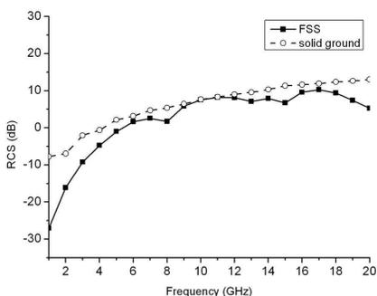
**Figure 9.** Comparison of simulated RCS of two reflectarrays with solid ground and FSS ground.
