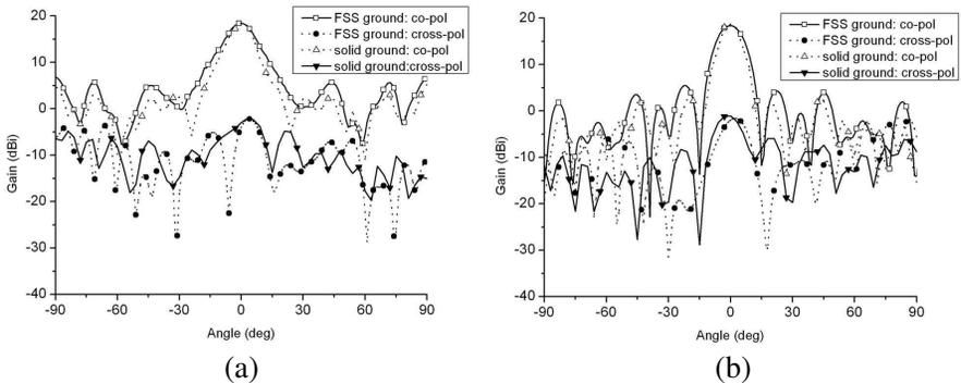
**Figure 8.** Measured radiation patterns for the reflectarray with FSS ground. (a)  $E$ -plane. (b)  $H$ -plane.
