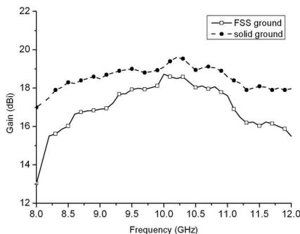
**Figure 10.** Measured gain versus frequency.
