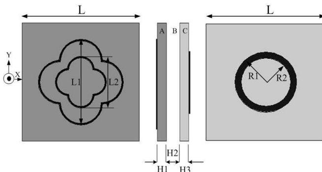
**Figure 1.** Geometries of the ring element of FSS and the top reflectarray element.
