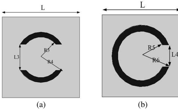
**Figure 3.** Geometries of (a) the split-ring and (b) C-ring.
