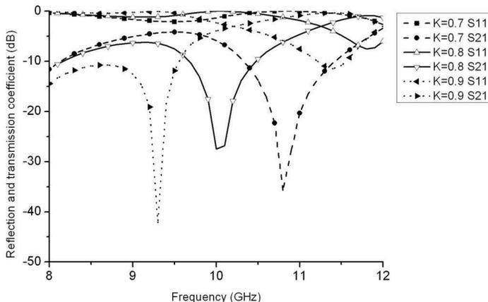
**Figure 2.** Reflection and transmission coefficients of the ring element of FSS with different  $K$ .
