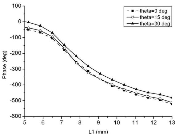
**Figure 6.** Phase responses of reflectarray element with FSS ground for different angles of incidence.
