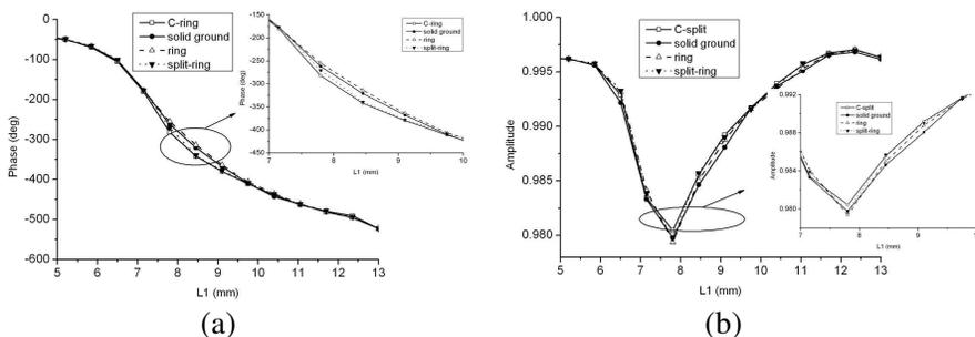
**Figure 5.** (a) Phase and (b) amplitude of the reflectarray element with the three types of FSS elements.
