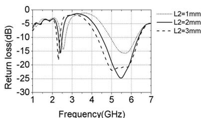
**Figure 8.** The effect of  $L_2$  on the return loss ( $L_1 = 11.9$  mm).
