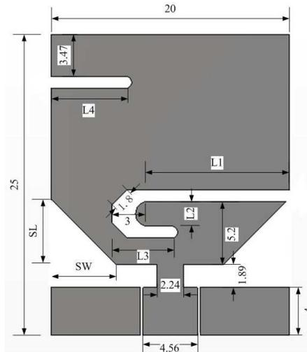
Figure 1. Top view of the antenna (unit: mm).
