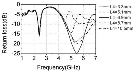
**Figure 5.** The influence of the top-left slot length on the return loss.
