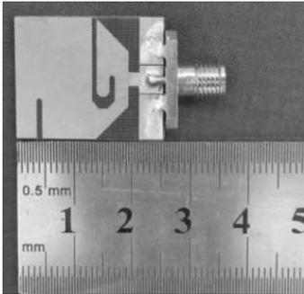
**Figure 3.** Prototype of the antenna.
