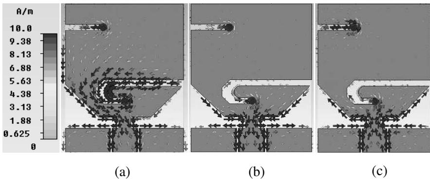
Figure 2. Current path, (a) 2.4 GHz, (b) 5.2 GHz, (c) 5.8 GHz.
