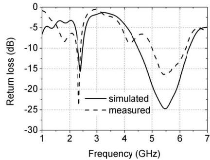
**Figure 4.** Measured and simulated return loss.
