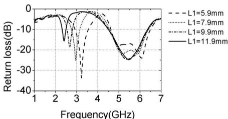
**Figure 7.** The effect of  $L_1$  on the return loss ( $L_2 = 2$  mm).
