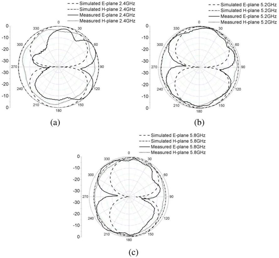
**Figure 9.** Measured and simulated radiation patterns, (a) 2.4 GHz, (b) 5.2 GHz, (c) 5.8 GHz.
