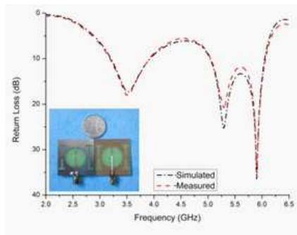
**Figure 5.** Simulated and Measured return losses of the antenna.
