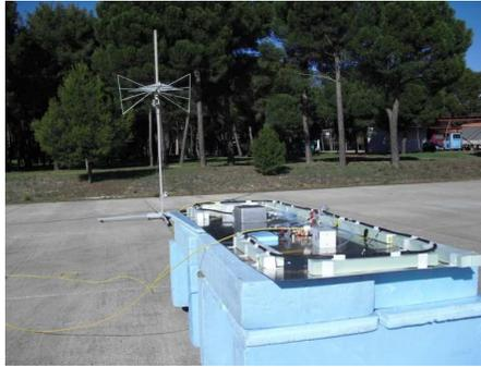
**Figure 1.** Experimental setup with the EMCO antenna at the INTA open-area test-site facility.
