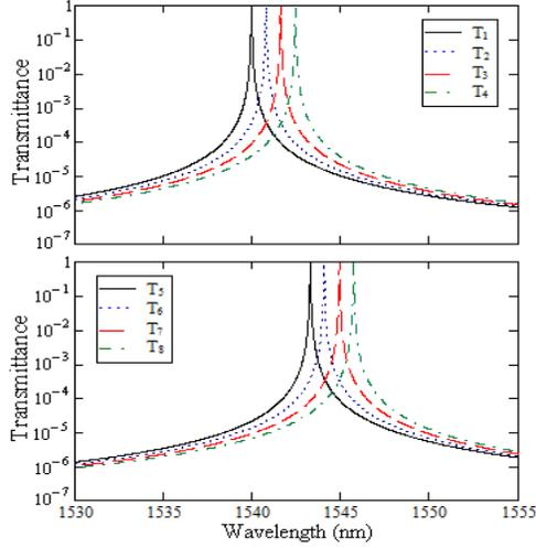
**Figure 3.** Transmission spectra of proposed structure at different temperature.
