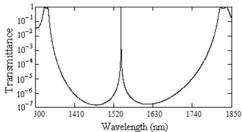
**Figure 2.** The defect mode for a PC with defect of  $[(\text{Si}/\text{ZnS})^5\text{Si}(\text{ZnS}/\text{Si})^5]$  at 300 K temperature.
