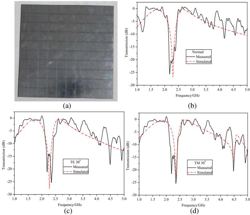
**Figure 5.** Experiment. (a) Prototype of the fabricated structure. (b) Simulated and measured results comparison with plane wave normal incidence. (c) Measured transmission curves with 30 degrees incident angle with TE polarization. (d) Measured transmission curves with 30 degrees incident angle with TM polarization.
