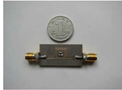
Figure 7. Photograph of the fabricated filter.
