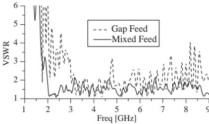
**Figure 3.** Comparison of measured VSWR between gap coupled LPMA and mixed feed LPMA.
