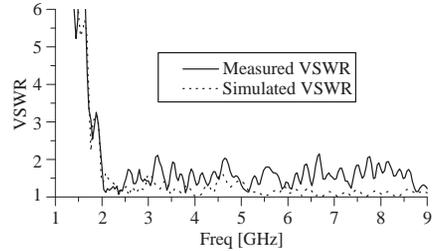
**Figure 4.** Measured and simulated VSWR of the proposed LPMA.
