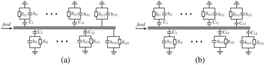
**Figure 2.** Equivalent circuit analysis. (a) Equivalent circuit of the proposed LPMA with mixed feed. (b) Equivalent circuit of the monolayer LPMA with gap feed.
