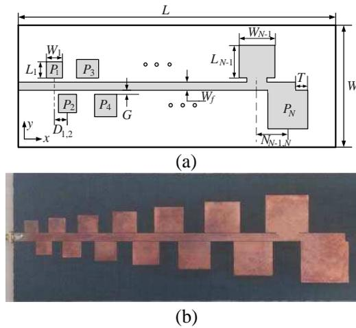
**Figure 1.** Configuration of the proposed LPMA. (a) Geometry of the proposed LPMA. (b) Photograph of the fabricated LPMA.
