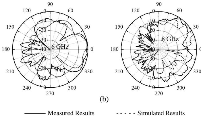
**Figure 7.** Measured and simulated radiation patterns at different frequencies. (a)  $xz$  plane. (b)  $yz$  plane.
