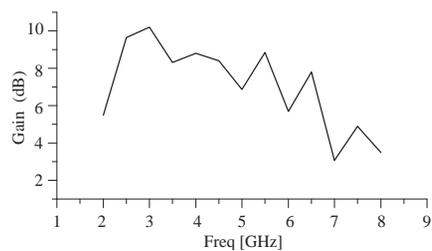
**Figure 6.** Measured gain of the proposed LPMA.
