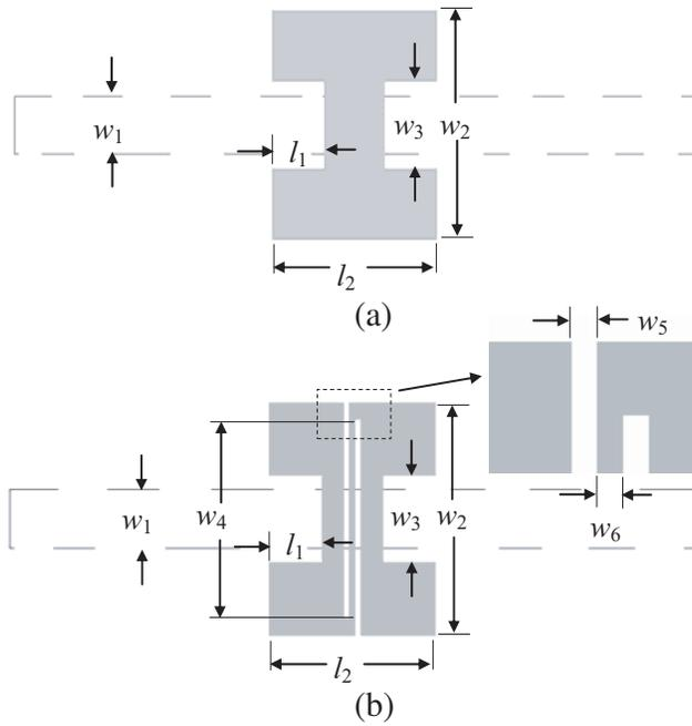
**Figure 1.** (a) Structure of the traditional DGS pattern and (b) the proposed DGS pattern.
