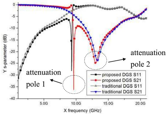
**Figure 2.** Simulated  $S$ -parameters of the traditional DGS and the novel DGS.
