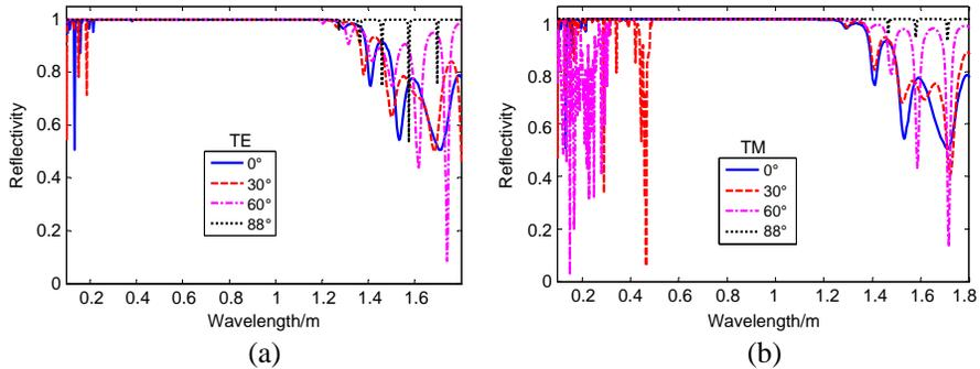
**Figure 4.** The calculated wavelength-dependent reflectance at four distinct incident angles of  $0^\circ$ ,  $30^\circ$ ,  $60^\circ$  and  $88^\circ$ . Here the thickness change rates of  $\Delta d = \Delta d_1 = \Delta d_2 = 9 \text{ nm}$  is used. (a) For TE wave. (b) For TM wave.
