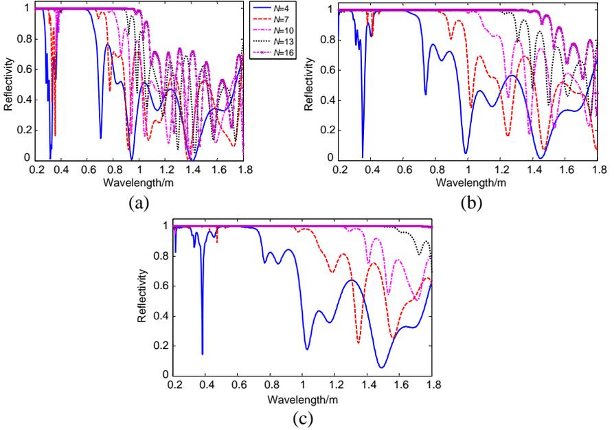
**Figure 3.** The calculated wavelength-dependent reflectance at different numbers of periods  $N = 4, 7, 10, 13$  and  $16$ , respectively. The same thicknesses rate of superconductor and dielectric layers is used, and the normal incidence is  $\theta = 0^\circ$ . (a) For  $\Delta d = \Delta d_1 = \Delta d_2 = 3$  nm. (b) For  $\Delta d = \Delta d_1 = \Delta d_2 = 6$  nm. (c)  $\Delta d = \Delta d_1 = \Delta d_2 = 9$  nm.
