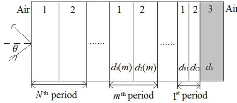
**Figure 1.** An  $N$ -period graded superconductor-dielectric periodic multilayer structure, in which layer 1 is the superconductor, layer 2 is the dielectric, and layer 3 is the glass substrate. The wave is incident in free space of region 0, and the region behind the substrate is also free space.
