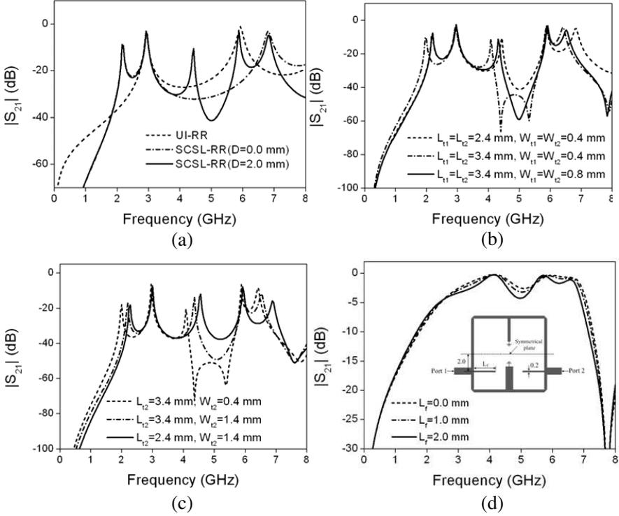
**Figure 2.** Frequency responses of the SCSL-RR circuit. (a) UI-RR and SCSL-RR. (b) Varied sizes of the two dissimilar stubs. (c) Varied sizes of one stub under  $L_{t1} = 3.4$  mm and  $W_{t1} = 0.4$  mm. (d) Varied stub length,  $L_f$ , in connection to the two tapped feed lines (unit: mm).
