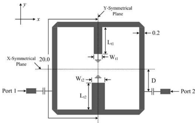
**Figure 1.** Schematic of the proposed SCSL-RR (unit: mm).
