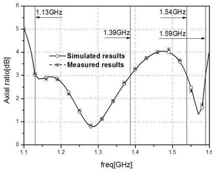
**Figure 9.** Comparison between the simulated and measured axial ratio of the proposed antenna.
