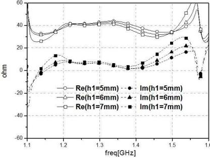
**Figure 2.** Simulated input impedance of the proposed antenna as the height of the  $L$ -probe feeds varies,  $h_1 = 5$  mm, 6 mm and 7 mm.
