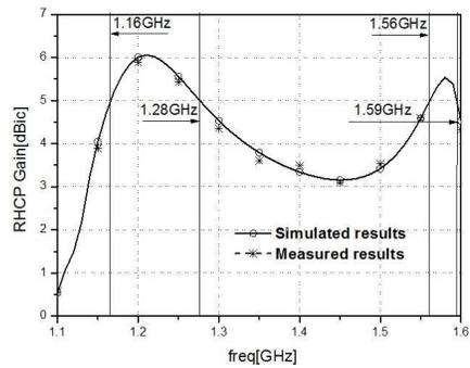
**Figure 10.** Comparison between the simulated and measured gain of the proposed antenna.
