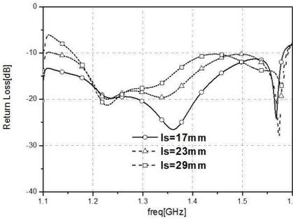
**Figure 4.** Simulated return loss of the proposed antenna as the length of  $L$ -probe feeds varies:  $l_s = 17$  mm, 23 mm and 29 mm.
