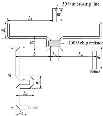
**Figure 6.** The Wilkinson power divider with two outputs having a 90° phase shift for feeding the proposed antenna.
