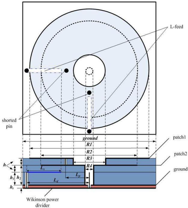
**Figure 1.** Geometry of the proposed antenna showing from top and side view.
