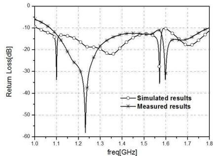
**Figure 7.** Comparison between the simulated and measured return loss of the proposed antenna.
