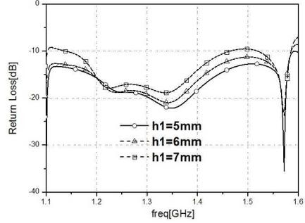
**Figure 3.** Simulated return loss of the proposed antenna as the height of the  $L$ -probe feeds varies,  $h_1 = 5$  mm, 6 mm and 7 mm.
