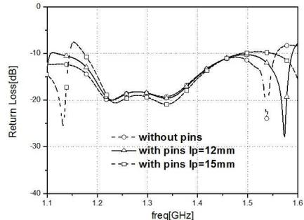
**Figure 5.** Simulated return loss of the proposed antenna with the effect of the shorted pins.
