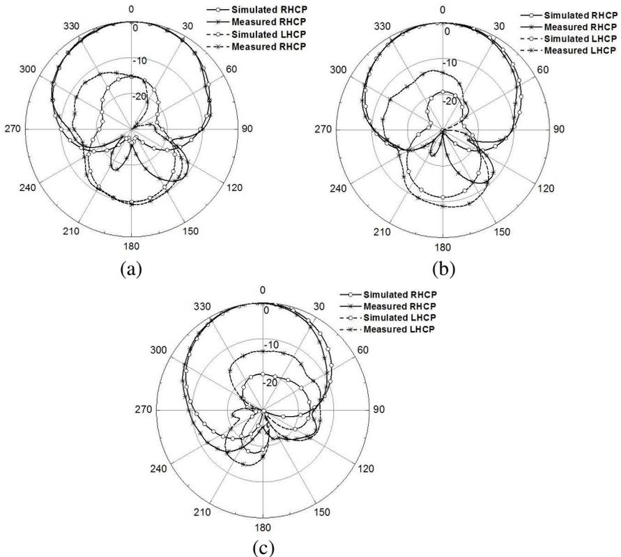
**Figure 8.** Comparison between the simulated and measured radiation patterns of the proposed antenna. (a) 1.176 GHz, (b) 1.227 GHz and (c) 1.575 GHz.
