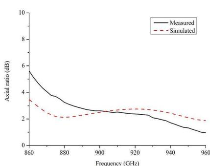
**Figure 8.** Simulated and measured axial ratio of the proposed antenna.
