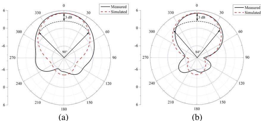
**Figure 6.** Simulated and measured radiation pattern of the proposed antenna. (a)  $\Phi = 0^\circ$ . (b)  $\Phi = 90^\circ$ .
