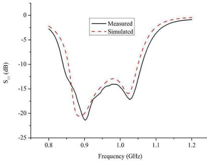
**Figure 4.** Simulated and measured  $S_{11}$  of the proposed antenna.
