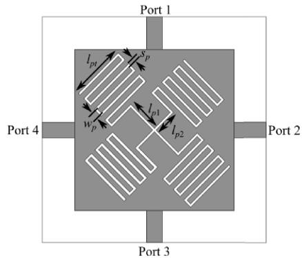
**Figure 3.** Configuration of the coupler.
