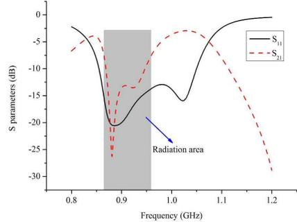
**Figure 5.** Simulated  $S$  parameters of the proposed antenna.
