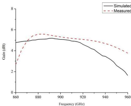
**Figure 7.** Simulated and measured gain of the proposed antenna.
