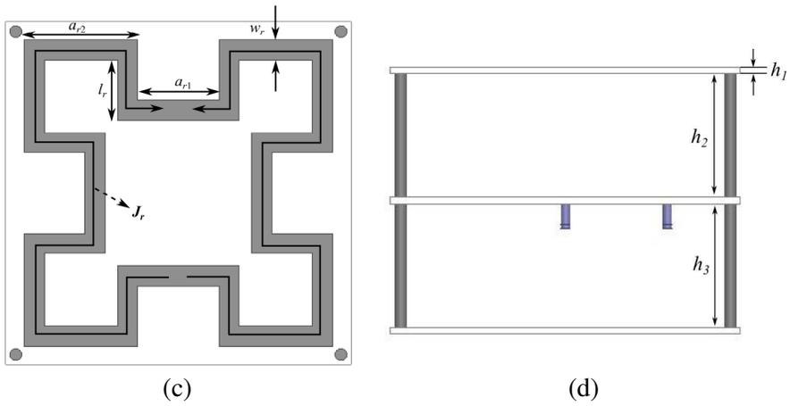
**Figure 1.** Configuration of the proposed antenna. (a) Director. (b) Driven element. (c) Reflector. (d) Cross view.
