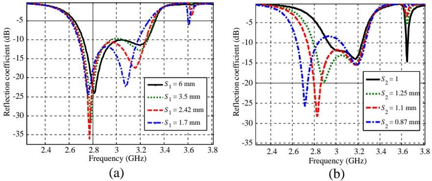
**Figure 3.** Computed reflection coefficient of the proposed antenna with one parasitic element ( $a = 18$ ,  $b = 18$ ,  $h = 8.9$ ,  $L_{slot} = 20$ ,  $w_a = 2$ ,  $d = 8$ ,  $l = 5.25$ ,  $\epsilon_r = 35.9$ ). (a) Different  $S_1$  lengths when  $S_2 = 1$  mm. (b) Different  $S_2$  lengths when  $S_1 = 3$  mm.
