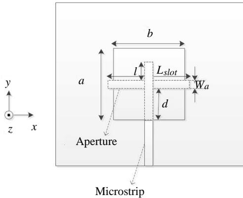
**Figure 1.** Geometry of the aperture coupled dielectric resonator.
