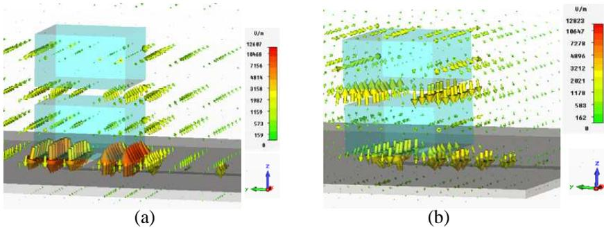
**Figure 2.** Electric field distribution of the proposed antenna. (a) 2.8 GHz. (b) 3.2 GHz.
