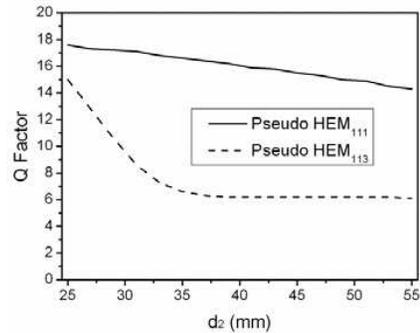
**Figure 7.**  $Q$  factors of the pseudo  $HEM_{111}$  and  $HEM_{113}$  modes of the one-step stair-shaped DR as a function of  $d_2$  ( $d_1 = 25$  mm,  $h_1 = h_2 = 10$  mm).
