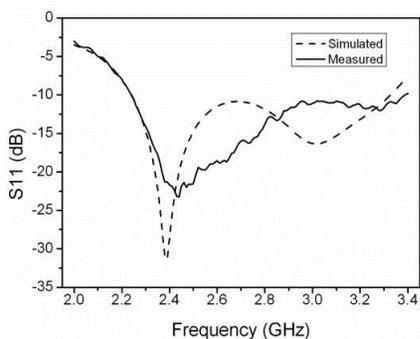
**Figure 9.** Simulated and measured return losses of the slot coupled one-step stair-shaped DRA.
