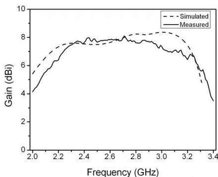
**Figure 11.** Measured gain of the slot coupled one-step stair-shaped DRA.
