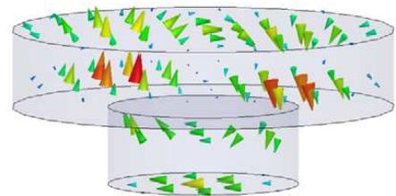
**Figure 5.**  $H$ -field of the second lowest order broadside mode in the second DR (the DR is mounted on the ground plane).
