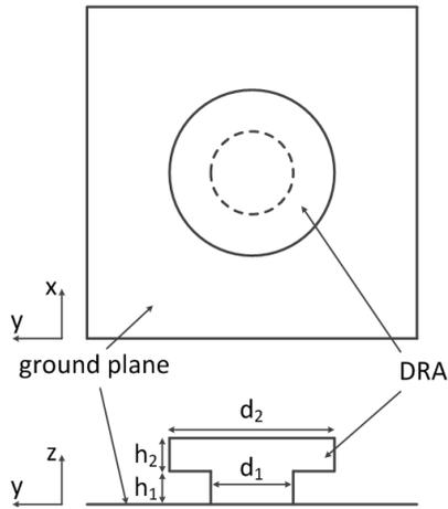
**Figure 1.** Geometry of the one-step stair-shaped DR placed on a ground plane.
