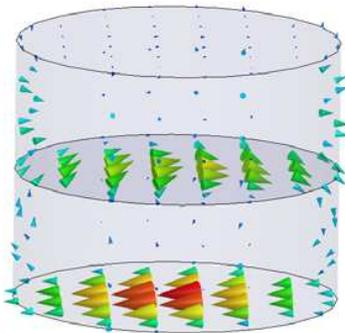
**Figure 4.**  $H$ -field of the second lowest order broadside mode in the first DR (the DR is mounted on the ground plane).
