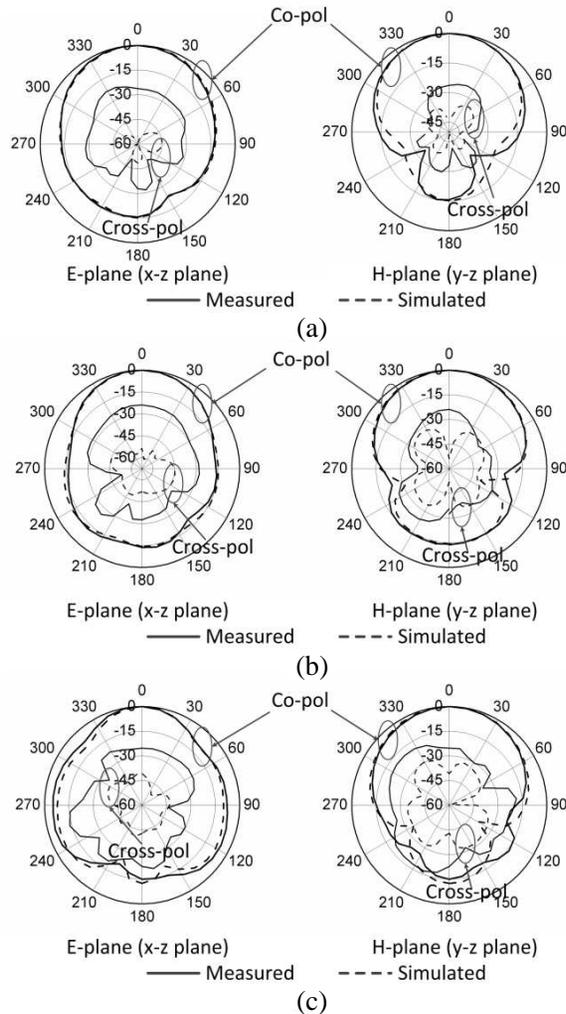
**Figure 12.** Measured radiation patterns of the slot coupled one-step stair-shaped DRA. (a)  $f = 2.3$  GHz; (b)  $f = 2.8$  GHz; (c)  $f = 3.3$  GHz.
