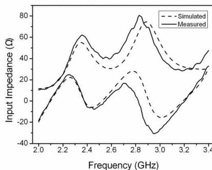
**Figure 10.** Simulated and measured input impedances of the slot coupled one-step stair-shaped DRA.
