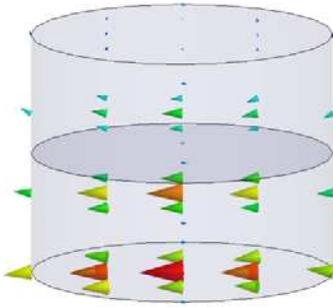
**Figure 2.**  $H$ -field of the fundamental broadside mode in the first DR (the DR is mounted on the ground plane).
