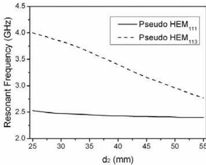
**Figure 6.** Resonant frequencies of the pseudo  $HEM_{111}$  and  $HEM_{113}$  modes of the one-step stair-shaped DR as a function of  $d_2$  ( $d_1 = 25$  mm,  $h_1 = h_2 = 10$  mm).
