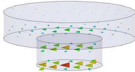
**Figure 3.**  $H$ -field of the fundamental broadside mode in the second DR (the DR is mounted on the ground plane).
