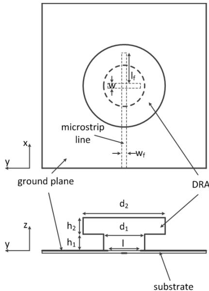
**Figure 8.** Geometry of the slot coupled one-step stair-shaped DRA.
