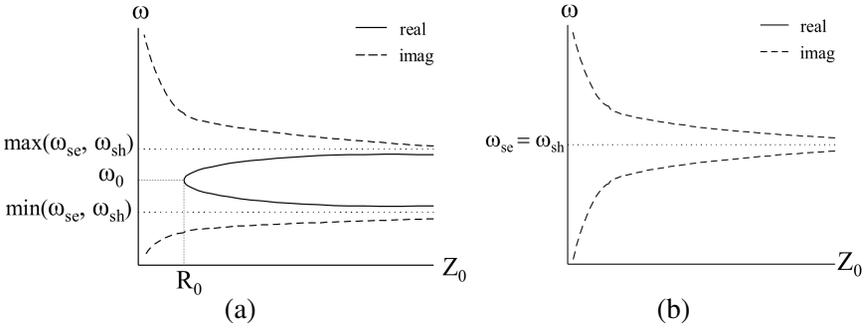
**Figure 3.** Characteristic impedances of the modified CRLH unit cell: (a)  $\omega_{se} \neq \omega_{sh}$ , and (b)  $\omega_{se} = \omega_{sh}$ .
