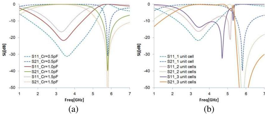
**Figure 4.** LC implementation of the UWB BPF with the modified CRLH structure: (a) single unit cell characteristics with different  $C_R$ 's, and (b) multiple unit cell characteristics with  $C_R = 1$  pF.
