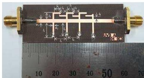
**Figure 5.** Photograph of the fabricated UWB BPF.
