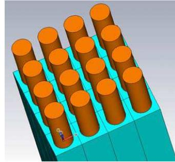
**Figure 11.** Layout of simple cubic pattern for gold nanorods on top of fiber endface.
