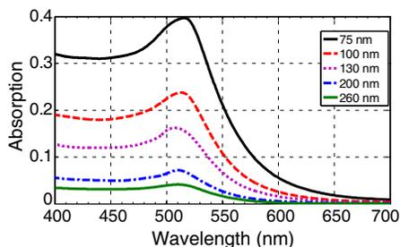
**Figure 4.** Absorption spectra of single-layered pattern with six neighbor nanospheres. The diameter of the nanoparticlespheres was 50 nm, and the center-to-center distance of the nanostructure was sampled between 75 nm to 260 nm.
