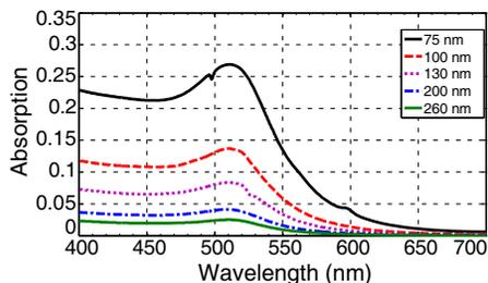
**Figure 2.** Absorption spectra of single-layered pattern with four neighbor nanospheres. The diameter of the nanospheres was 50 nm and the center-to-center distance of the nanostructure was sampled between 75 nm to 260 nm.
