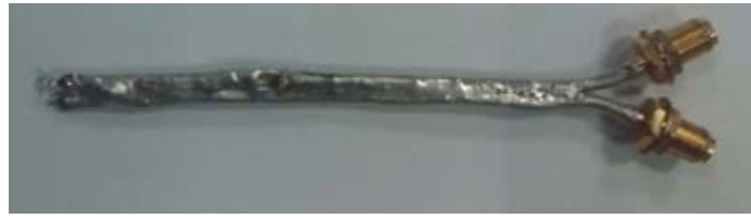
Figure 5. A fabricated fixture connecting the tag antenna to the network analyzer.
