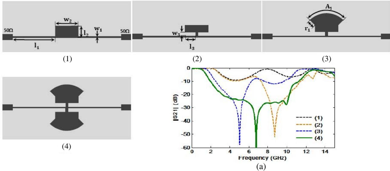
**Figure 5.** Mirrored series-resonant branch loaded by radial stub resonator design process and simulations. (1) 3-pole LPF using open-circuited stub, (2) series-resonant branch, (3) series-resonant branch loaded by radial stub, and (4) mirrored structure, (a)  $S_{21}$  simulations.
