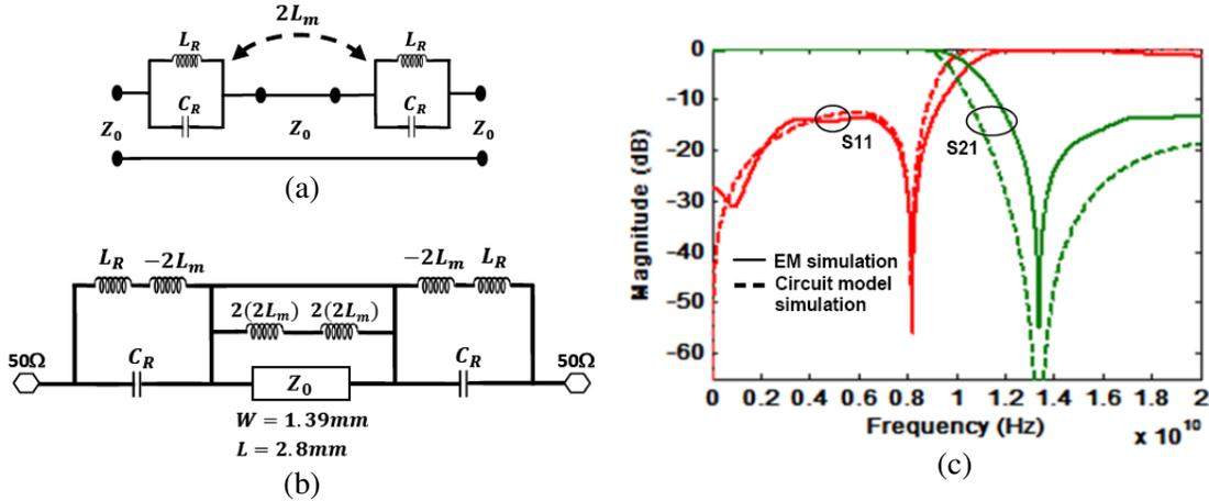
**Figure 4.** Coupled CDGS filter, (a) the simple equivalent circuit, (b) the novel detailed equivalent circuit model for the magnetically coupled CDGS resonators, (c) fall wave electromagnetic simulation compared with circuit model simulation (in case  $s = 0.4$  mm).
