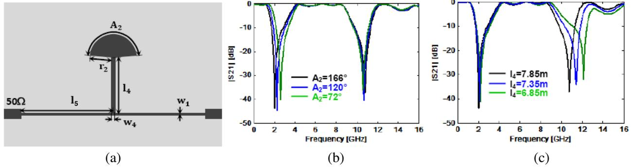
**Figure 6.** High impedance lines loaded by radial stub resonator, (a) structure, (b) transfer characteristics for different  $A_2$  ( $l_4 = 7.85$  mm), (c) transfer characteristics for different  $l_4$  ( $A_2 = 166^\circ$ ).
