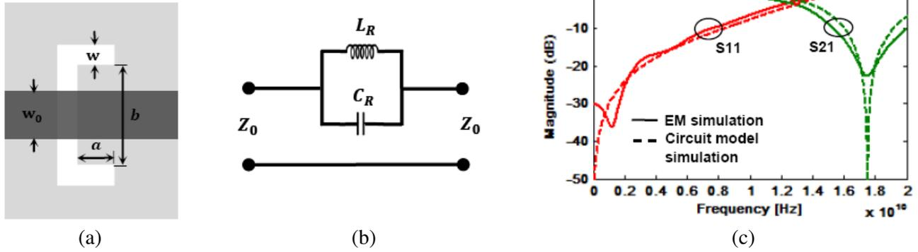
**Figure 2.** C-shape DGS unit, (a) structure, (b) equivalent circuit model, (c) circuit and EM simulations.
