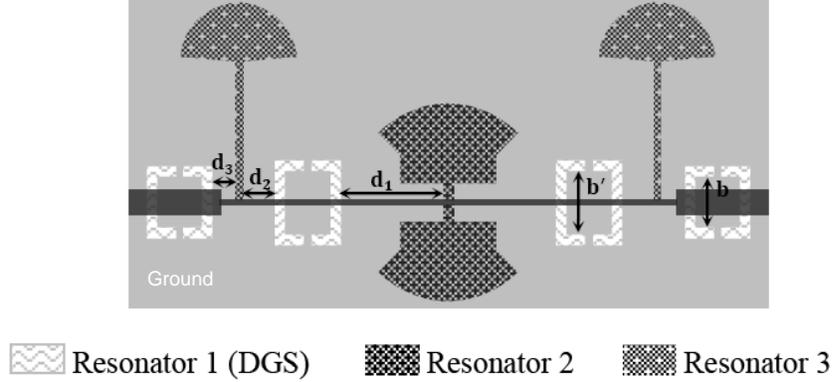
**Figure 1.** Layout of resonators used in the LPF design. Grey zones represent the metallization of microstrip: the dark shade denotes the top layer, while the light shade represents the ground.
